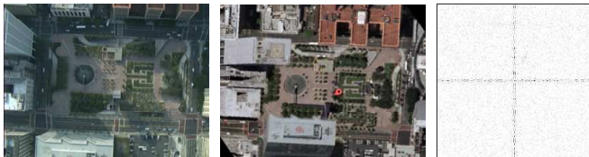
Fig. 2. Video image, rotated and scaled satellite image and phase correlation map. The true registration is at (15,29) and the map ranges from -100 to 100 in both x and y directions.
