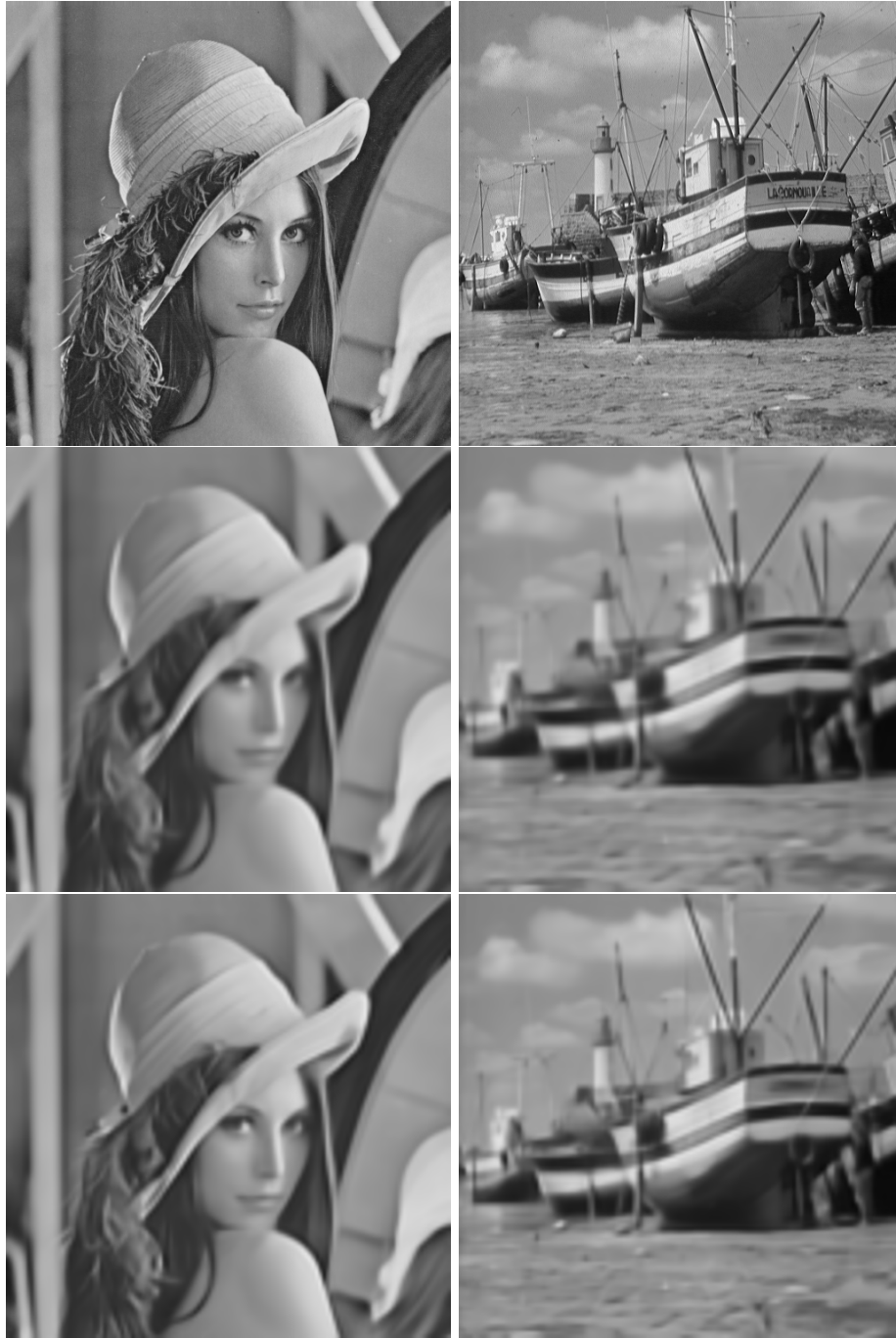
Figure 2.4: Reconstructed images. Top: original images. Middle: images reconstructed using LARS. MSE_{Lena} = 0.0027, MSE_{Boat} = 0.0035 . Bottom: images reconstructed using FSA. MSE_{Lena} = 0.0024, MSE_{Boat} = 0.0031 .
