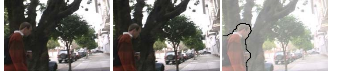
Figure 9. Motion segmentation where both camera and person are moving. I_1 (left), I_2 (middle), segmentation (right).
