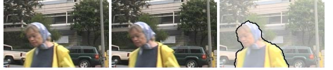
Figure 8. Motion segmentation where both camera and person are moving. I_1 (left), I_2 (middle), segmentation (right).
