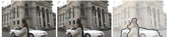
Figure 11. Motion segmentation with moving camera, car and people. I_1 (left), I_2 (middle), segmentation (right).
